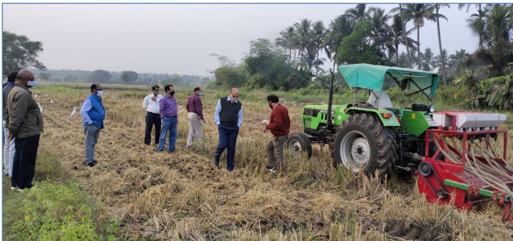
Field evaluation of the developed tractor operated straw chopper cum seeder in Farmers' field, Village-Resinga, Nimapara, Puri
