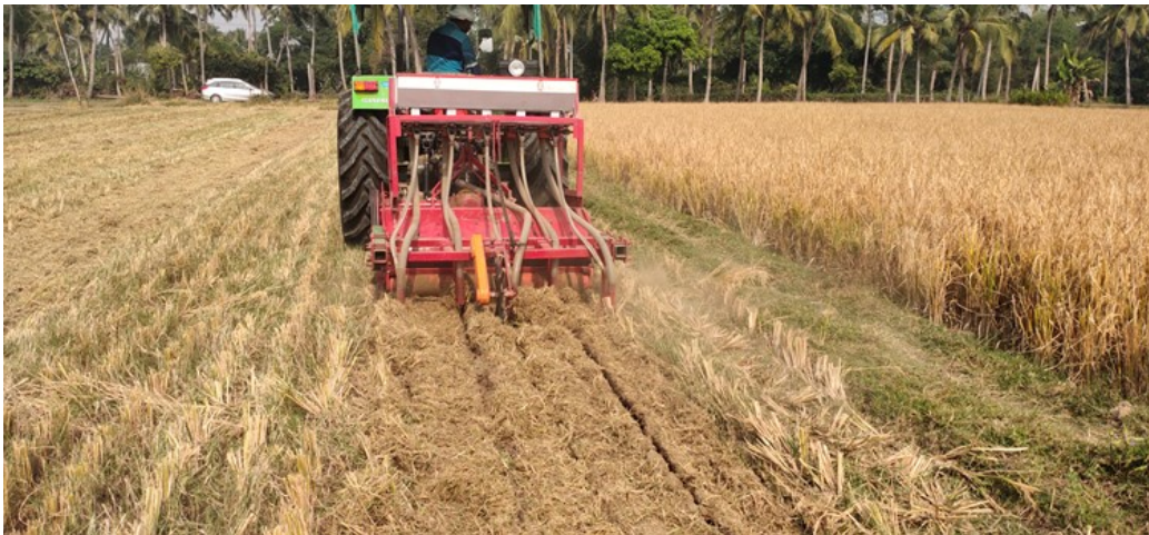
Field evaluation of the developed tractor operated straw chopper cum seeder in Farmers' field, Village-Resinga, Nimapara, Puri
